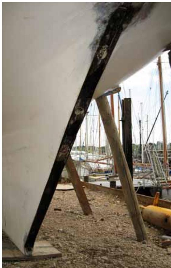
So with the rudder tube returned to me in four pieces the next quandary was how to make good the repair, and try and work out what had caused the problem in the first place. Most baffling was that having had the stock out in 1988 and re-assembled it with copious amounts of Keenol grease why had it seized, considering the same parts had lived harmoniously together for the first sixty-two years of the boat's life.
