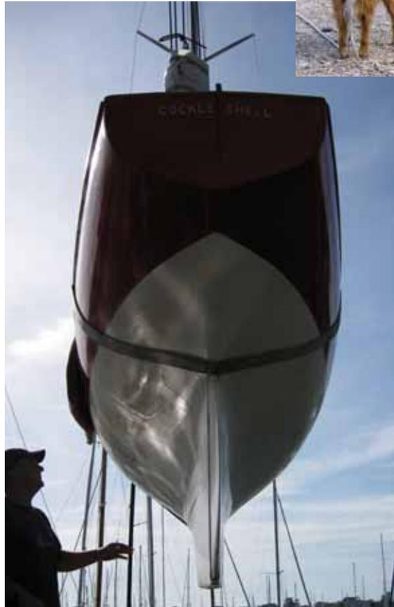
With the two part rudder tube now sealed in place and all the parts offered up it was time for final reassembly.
